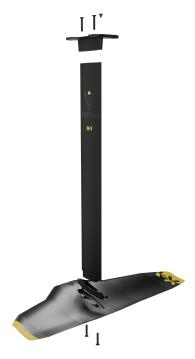
Install the base onto the flat-sided (non-machined) mast end with 2 M8 x 40 mm screws.
