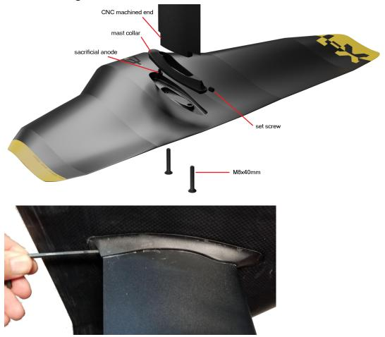
Set the collar into the wing and tighten two M8 x 40mm screws. Do not use shorter M8 screws. Use Tefgel. Check all screws before every use.
